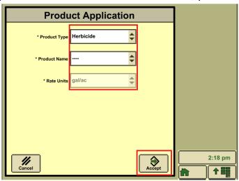
13. If you are doing a Tank Mix, you need to switch the Product Application Type to Tank Mix. Then you will have to make a new Tank Mix or use an existing mix. To make a new Tank Mix, a person would have to press the Add Carrier button.
