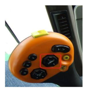
6. When header is at desired elevation press the "F" Button to save the current feederhouse height for the Record Stop Height. The percentage will change after the "F" button is pressed.
