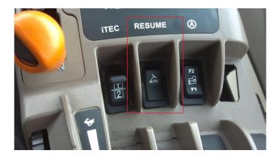
11. Once you press the "Resume or Auto" Button you will hear a beep noise and the AutoTrac Pie will turn green with a big A in the center of the pie. This means that AutoTrac is active.
