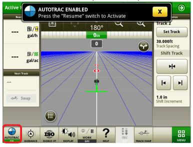
10. Drive the vehicle close to the AB Line and press "Resume or Auto" Switch to activate autotrac.
