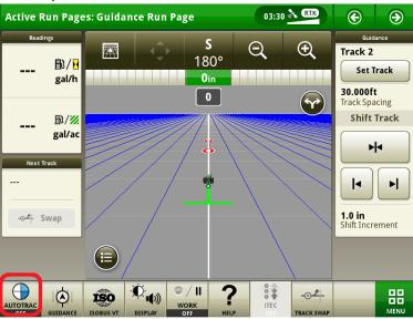
9. Press the AutoTrac Pie to enable the AutoTrac. After you do this, 3 pieces of the AutoTrac Pie should be filled in.
