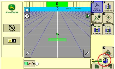
11. Get close to AB Line and press "Resume or Auto" Switch on Right Hand Console of Tractor.
