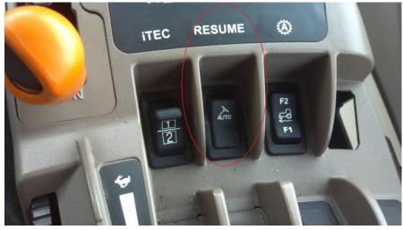
12. Once the Resume Switch is Pressed you will hear a noise and the Autotrac Pie turns Green with a big "A" in the center of it.
