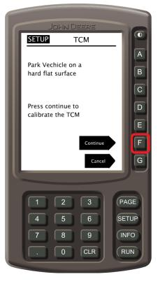
6. Turn the vehicle 180 degrees to face opposite direction and park vehicle so that fixed axle is equal to same reference point as Step 5. Once vehicle is at complete stop press "F" for "Continue".
