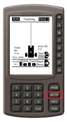
2. Press the "B" button for" StarFire Receiver".
